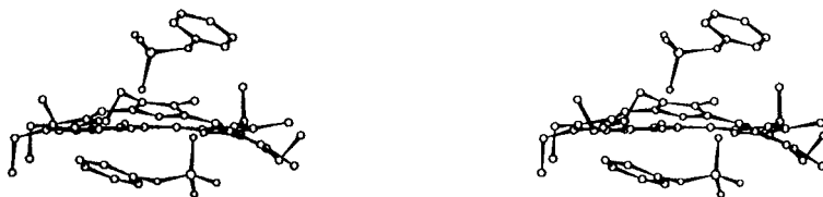
Figure 49. Single-crystal X-ray structure of the bis(phenylphosphate) salt of 276 . The anions are held at ~1.4 Å above and below the sapphyrin plane. 52 (Modified from ref 10.)
